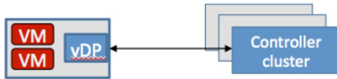
To gain scale the controller test will support 5,000 hypervisors and 100,000 logical ports. Ixia's IxVM will be the VM running within the hypervisors. There are two approaches to accommodate this level of scale: 1) deploy two 42 RU server racks with 60 VMs per server or 2) deploy the inception model (named after the movie *Inception*).
